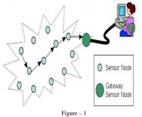
Wireless sensor networks find a variety of applications like robotic landmine detection, target tracking, environment protection, wildfire detection, home, traffic monitoring, for monitoring natural phenomenon etc. There may be three ways in which the application of a wireless sensor network may be divided. They are:
